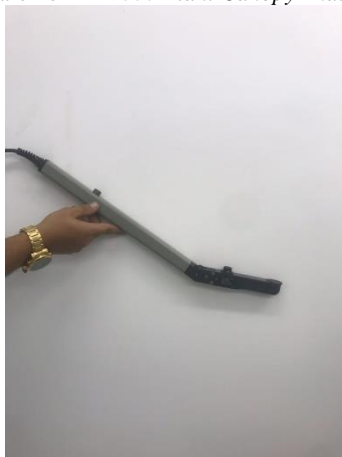
Figura 2: Aparelho LAI-2000 Plant Canopy Analyzer
